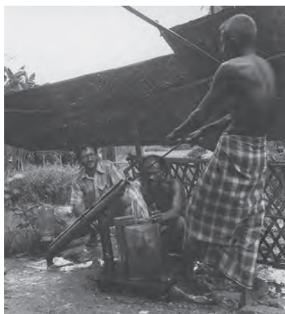
George Klassen of Calgary, Alberta (far left) designed and developed the rower pump in Bangladesh. The simple inexpensive irrigation pump was soon in use across Asia. Photo credit MCC.
