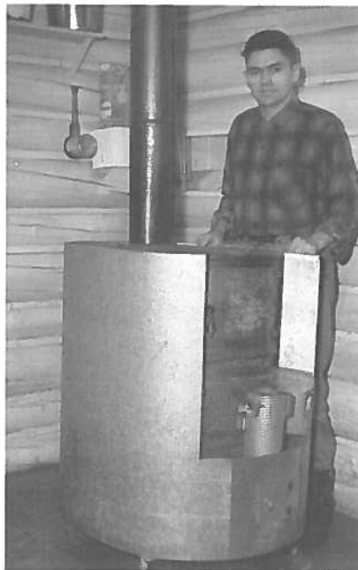
Henry with the stove he built from a large gas drum.
